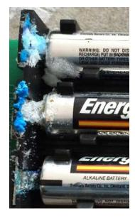
Figure 1: General Leakage Example (Not an Alcares Product)
