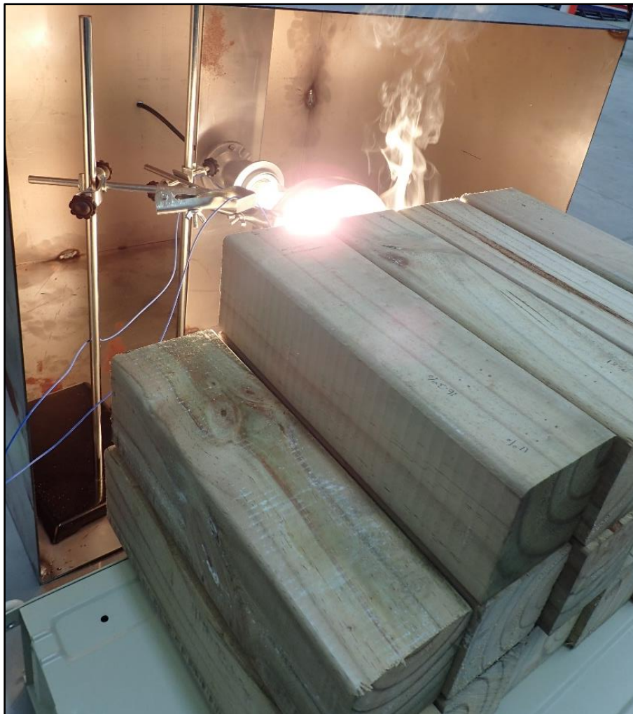
Figure 4 Lamp test set-up
