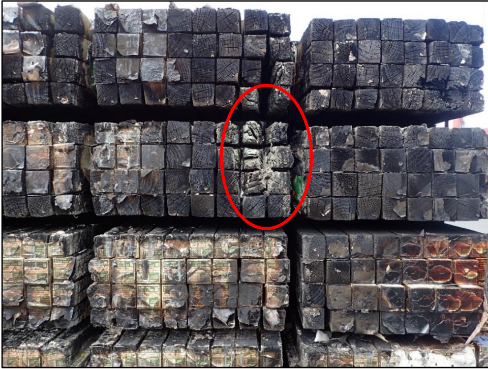
Figure 9 Timber packet showing origin of fire
