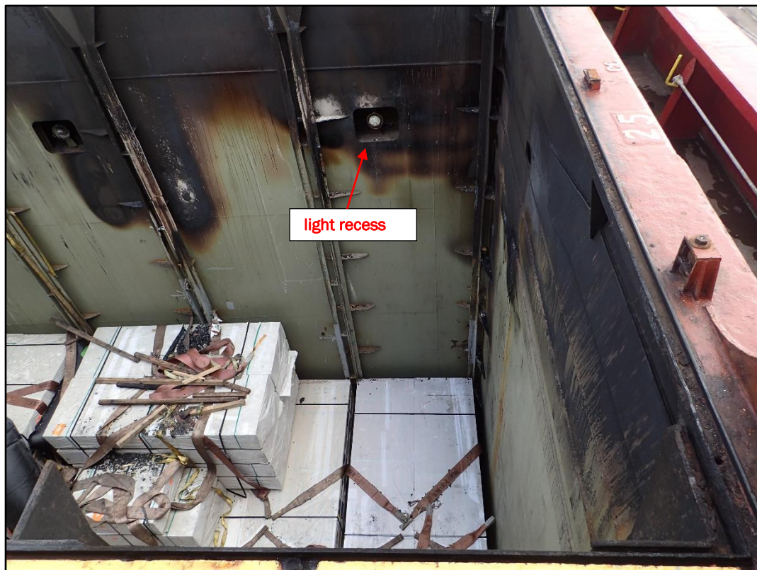
Figure 2 Remaining timber stowed in number 4 cargo hold after damaged timber had been removed
