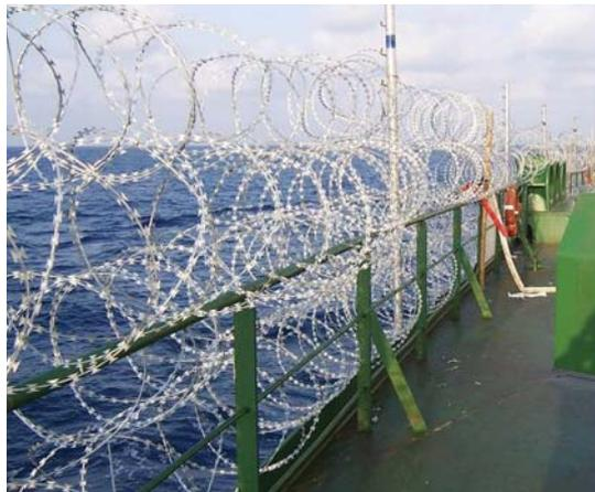
Concertina razor wire is recommended as the linked spirals make it the most effective barrier. Razor wire should be constructed of high tensile wire, which is difficult to cut with hand tools. Concertina razor wire coil diameters of approximately 730 mm or 980 mm are recommended.
