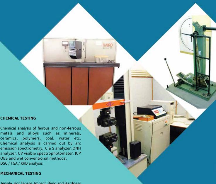
Chemical analysis of ferrous and non-ferrous metals and alloys such as minerals, ceramics, polymers, coal, water etc. Chemical analysis is carried out by arc emission spectrometry, C & S analyzer, ONH analyzer, UV visible spectrophotometer, ICP OES and wet conventional methods.
