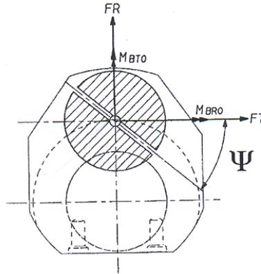
**Fig.6 : Crankpin section through the oil bore**
