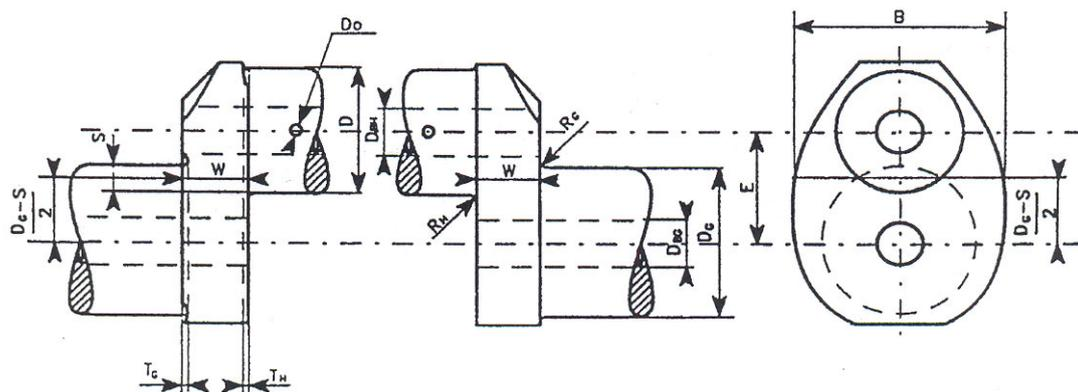
**Fig.7 : Crank dimensions**
