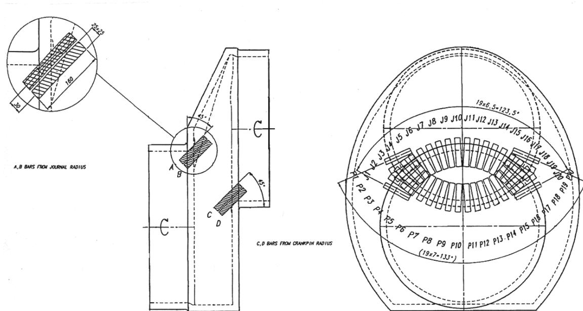
Figure 3.1. Specimen locations in a crank throw
