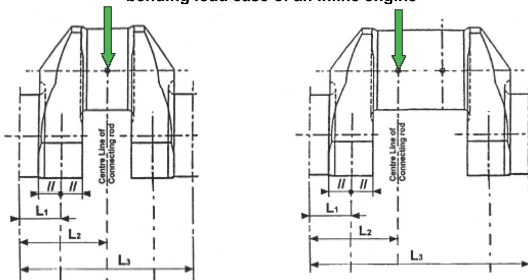
**Fig. 3.4 : Load applications for in-line and V-type engines**
