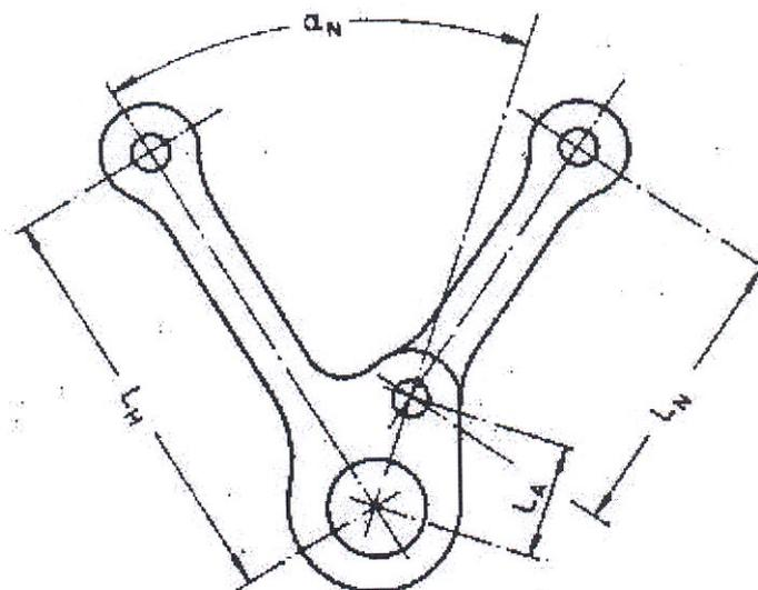
**Fig. 2 : Articulated-type connecting-rod**
