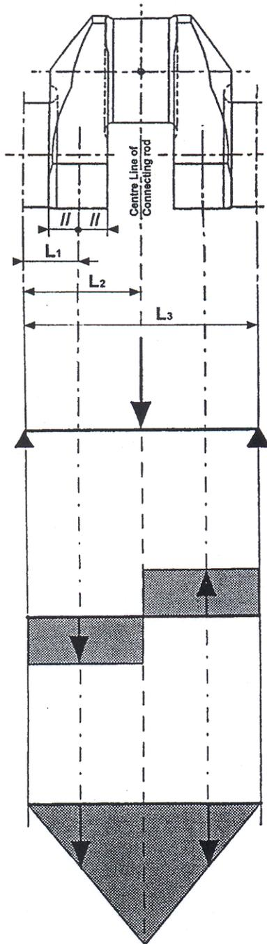
**Fig. 3 : Crankthrow for in line engine**
