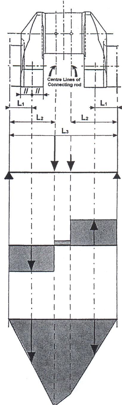
**Fig.4 : Crankthrow for Vee-engine with 2 adjacent Connecting-rods**
