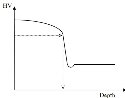
*Figure 4.1. Typical hardness as a function of depth. The arrows indicate the defined hardening depth. Note the indicated potential hardness drop at the transition to the core. This can be a weak point as local strength may be reduced and tensile residual stresses may occur.*
