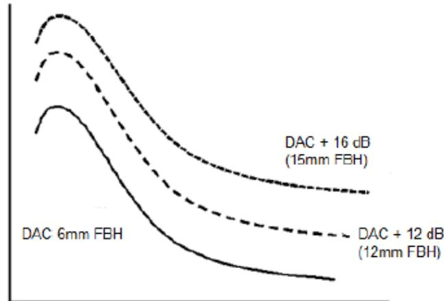
**Fig. 6.3.8: DAC curve produced from 6.0mm FBH reflector and DAC curves adjusted to represent equivalent 12.0mm and 15.0mm FBH reflectors.**
