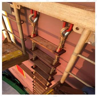
6.9. When a combination arrangement in use, the lower platform should be a minimum of 5 metres above sea level:
