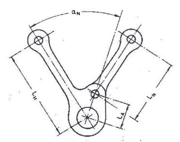
Fig. 2 : Articulated-type connecting-rod
