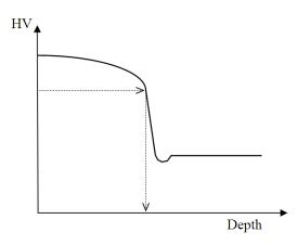
Figure 4.1. Typical hardness as a function of depth. The arrows indicate the defined hardening depth. Note the indicated potential hardness drop at the transition to the core. This can be a weak point as local strength may be reduced and tensile residual stresses may occur.
