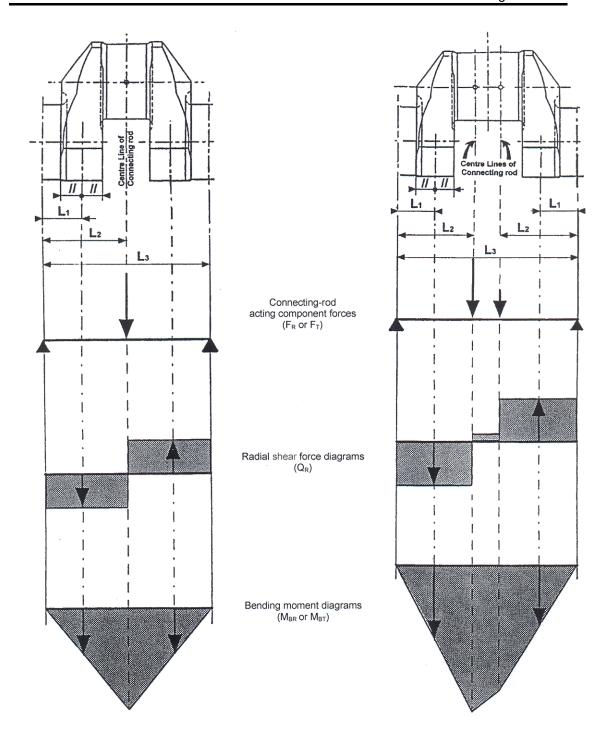
Fig. 3: Crankthrow for in line engine
