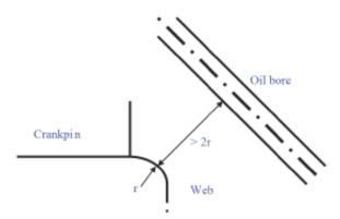
Fig.2.1: Oil bore proximity to fillet
