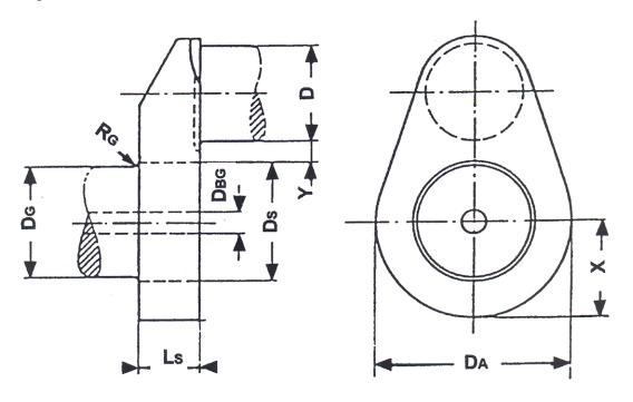
Fig.8: Crankthrow of semi-built crankshaft
