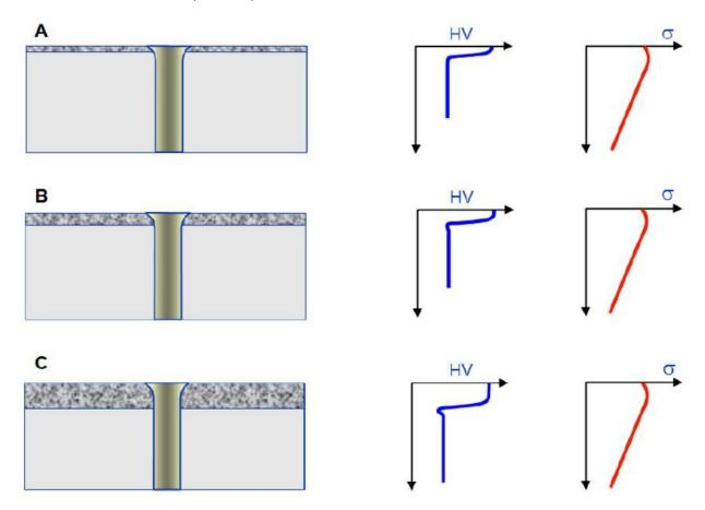
Figure 3.4. Stresses and hardness in induction hardened oil holes
