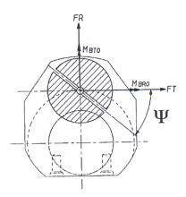
Fig.6: Crankpin section through the oil bore
