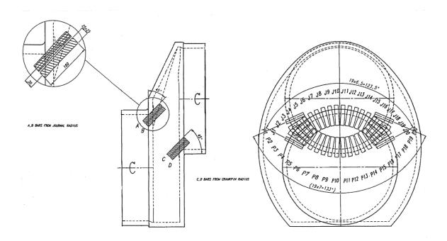
Figure 3.1. Specimen locations in a crank throw
