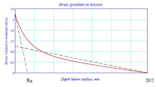
Figure 3.3. Torsional SCF in the crankpin fillet as a function of depth. The corresponding SCF for the journal fillet can be found by replacing  $R_{\rm H}$  with  $R_{\rm G}$  and D with  $D_{\rm G}$
