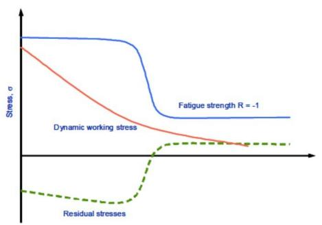
Figure 3.1. Stresses as functions of depth, general principles
