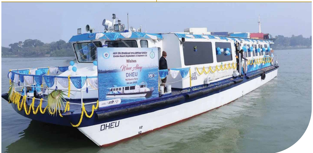
'Dheu,' the Next Generation Zero-Emission Electric Ferry built under (IRS) Guidelines for Battery - Powered Vessels, delivered by GRSE - Garden Reach Shipbuilders & Engineers Ltd. to the Government of West Bengal.
