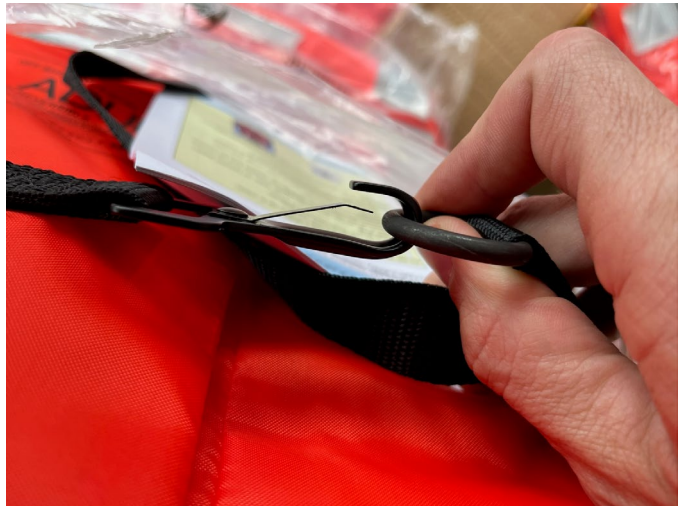
Example of a partially closed snap hook.
